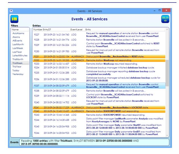
The program is fully integrated into the Main Viewer. When a user requests to view events associated with a specific system object, Main Viewer launches Event Viewer and displays the latest 1000 or so (depending on default filter settings) event log records (and alarms) associated with that object.
