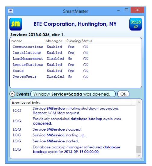
Each window is associated with one of system objects (subsystems) being monitored. In above case the window is associated with SmartMaster<sup>TM</sup> service, the top service, as described in previous section.
